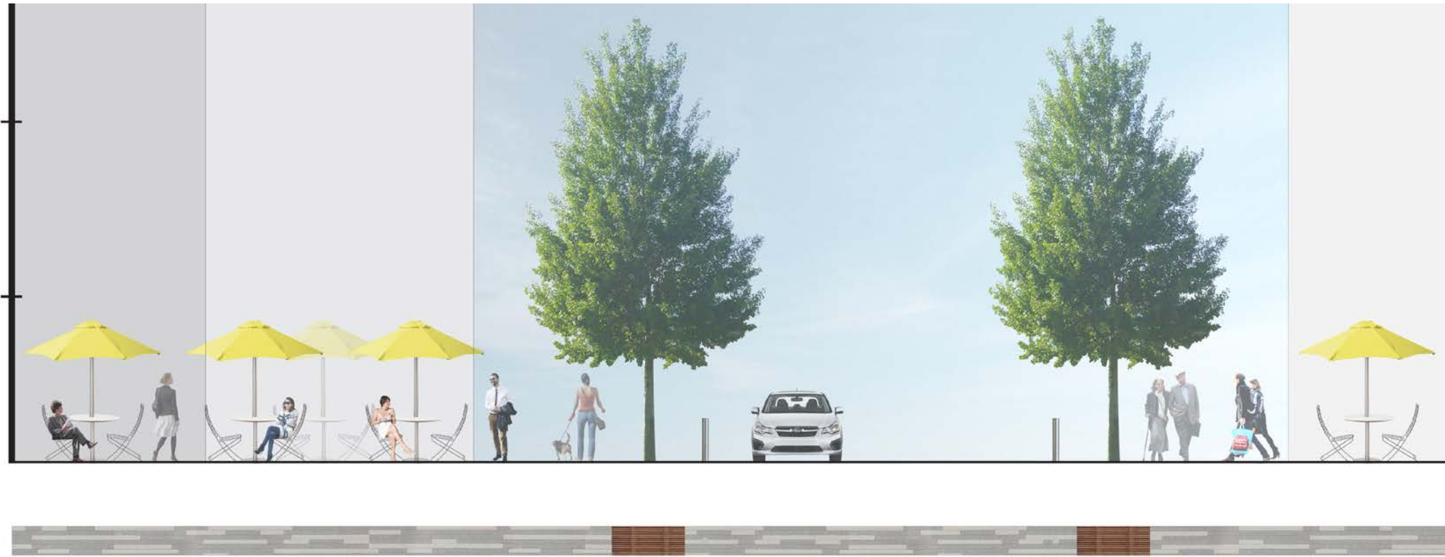
SECTION A-A: CURBLESS STREET
