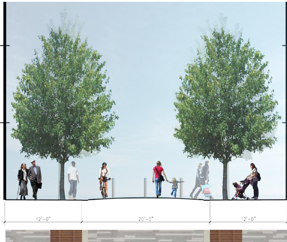
SECTION B-B': CURBLESS PEDESTRIAN STREET
