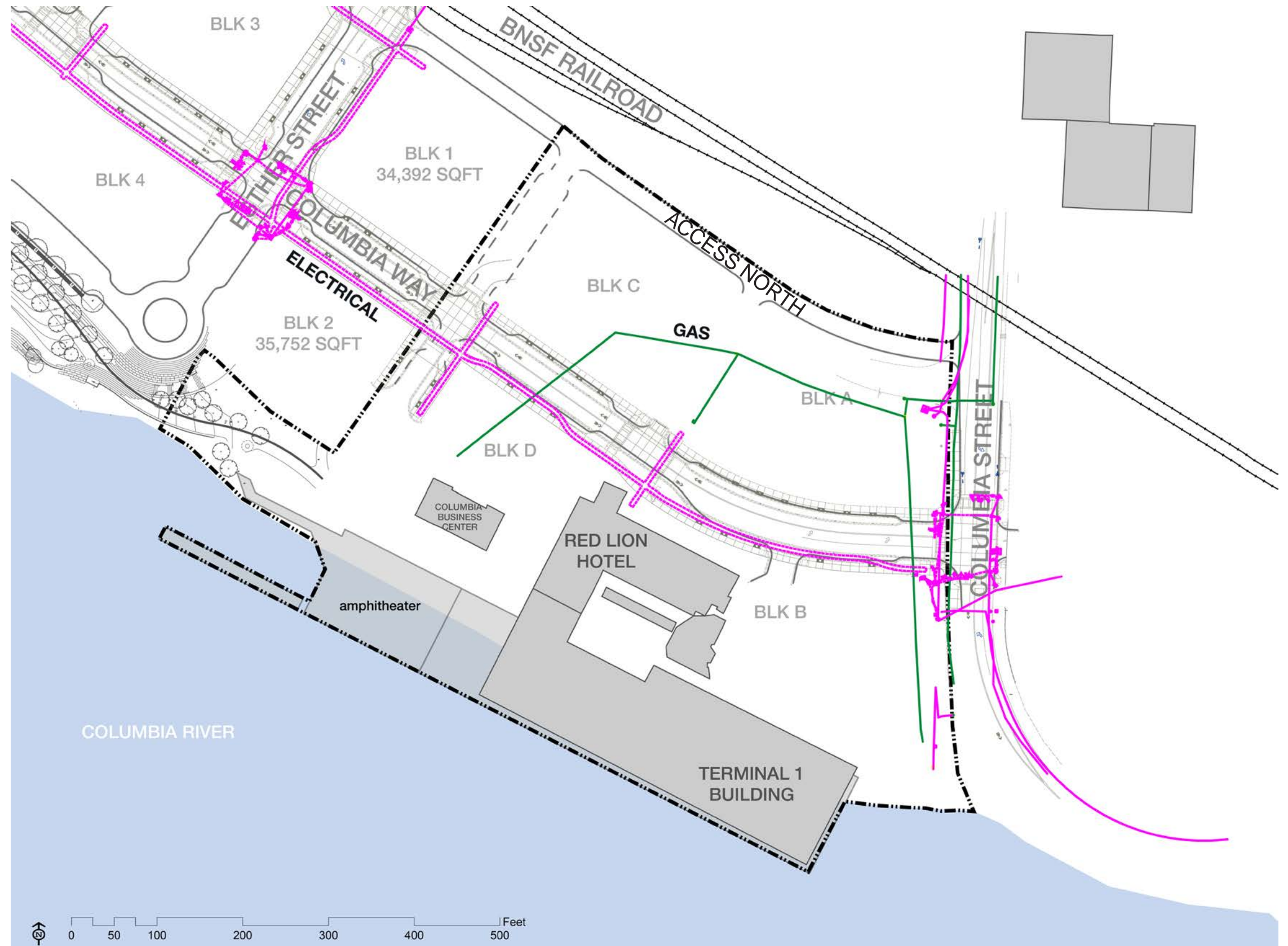
Figure 1.51 Existing Utilities: Electrical & Gas
