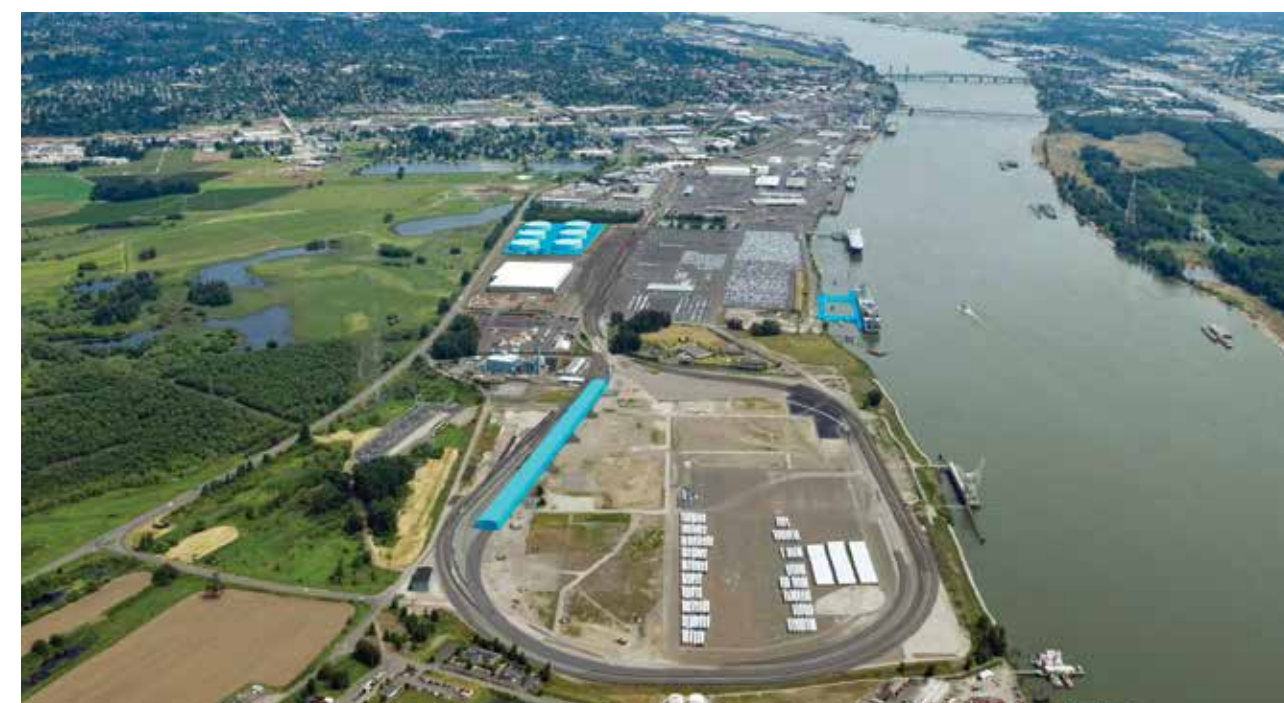
The proposed Vancouver Energy facility (highlighted in blue) consists of a covered transload area on the railroad tracks at Terminal 5, six storage tanks to the east and a loading area at two of the port's cargo berths.
