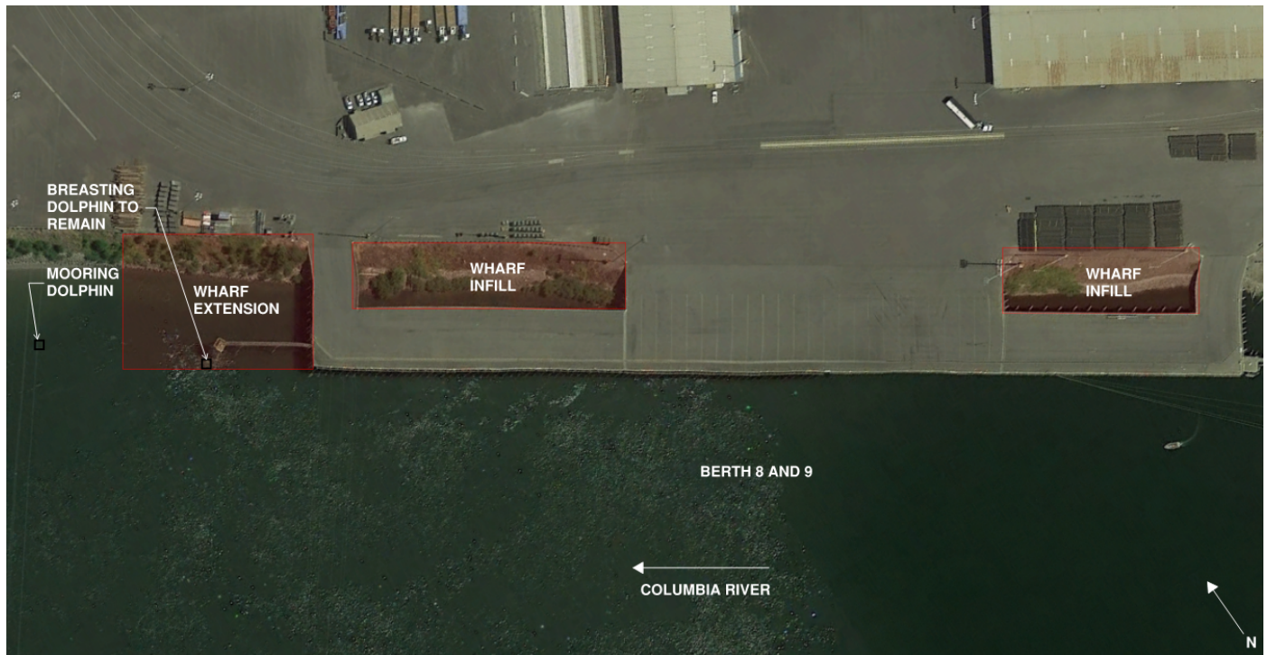
Figure 2. Proposed Wharf Extension and Infill (Preliminary)
